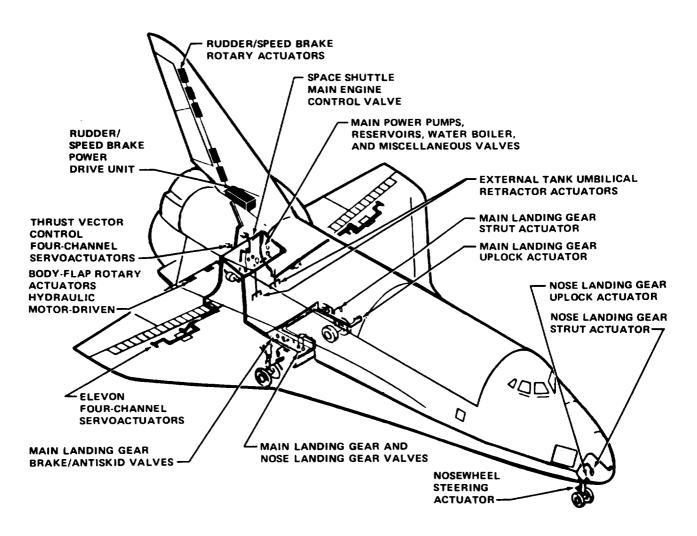
Figure 4-4.—Orbiter hydraulic system.
