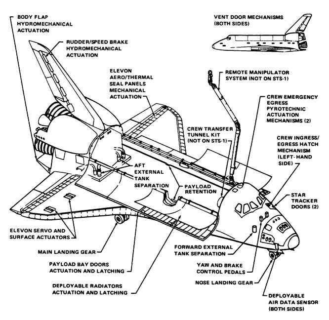
Figure 3-20.— Mechanical subsystems.
