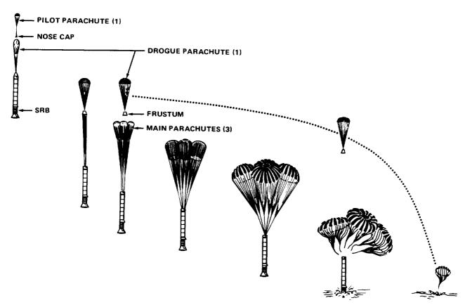
Figure 2-13.—SRB parachute deployment.
