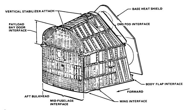
Figure 3-14.— Aft fuselage shell structure.
