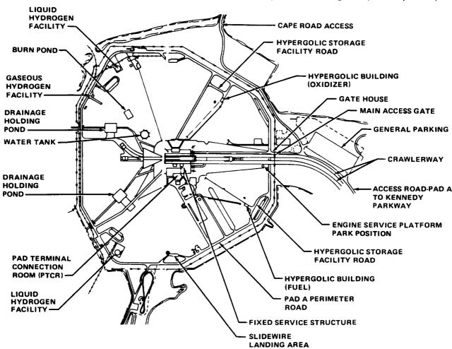
Figure 6-8.—Launch Pad 39-A surface arrangement.
