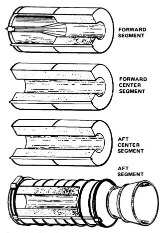
Figure 2-8.—Space Shuttle solid rocket motor.
