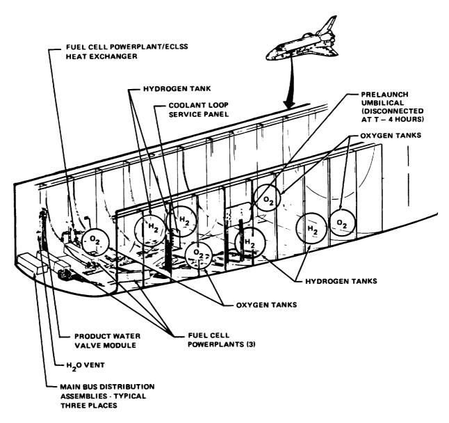
Figure 4-3.—Electrical power system.
