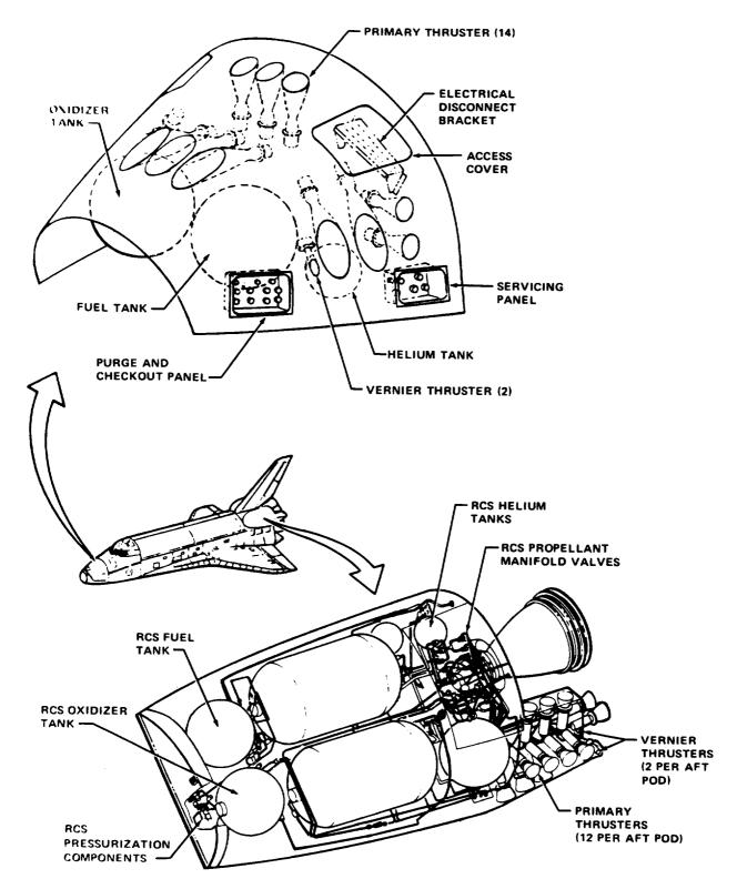
Figure 4-2.—Reaction control system.
