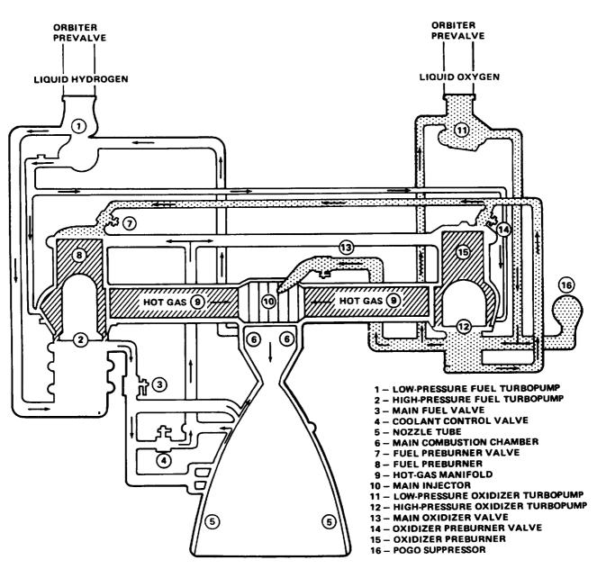
Figure 2-3.—SSME propellant flow schematic.
