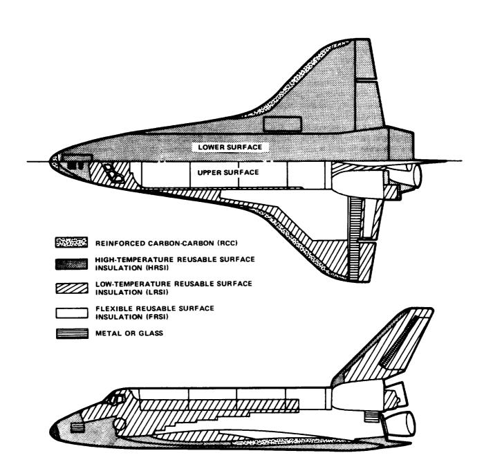
Figure 4-9.— Orbiter thermal protection system.
