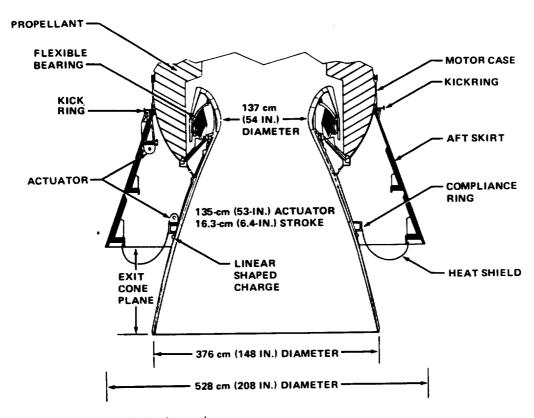
Figure 2-11.—Solid rocket motor nozzle.
