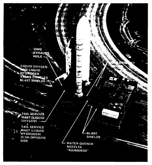
Figure 6-6.—Mobile Launcher Platform exterior view (108-KSC-79P-143).
