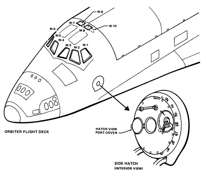
Figure 5-10.—Window shade and filter locations.
