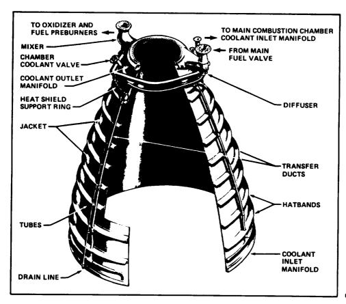
Figure 2-5.—SSME nozzle assembly.
