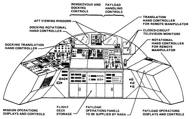
Figure 3-6.— Aft flight-deck configuration.
