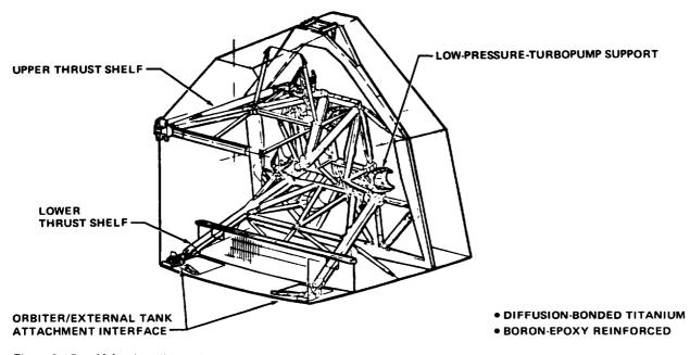
Figure 3-15.— Aft fuselage thrust structure.
