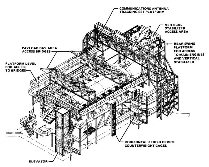
Figure 6-2.—Orbiter Processing Facility.
