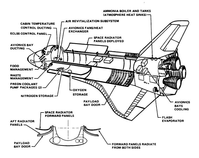
Figure 4-6.— Orbiter environmental control and life-support system.
