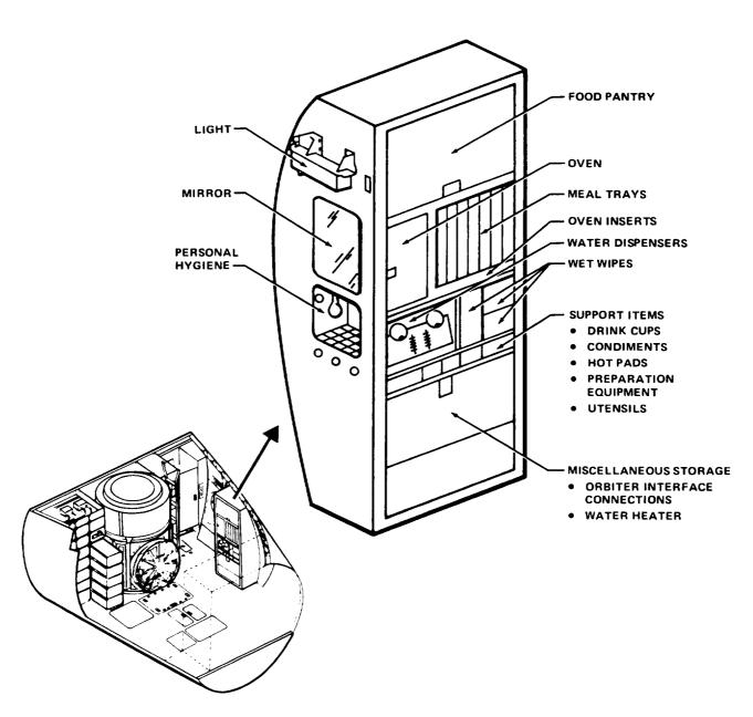
Figure 5-11.—Galley configuration (concept).
