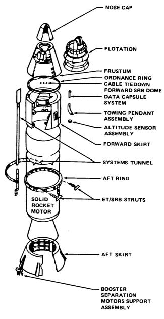
Figure 2-12.—SRB structural system (MSFC 776268A).
