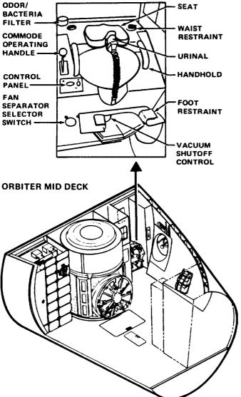
Figure 4-8.—Orbiter waste collection system.
