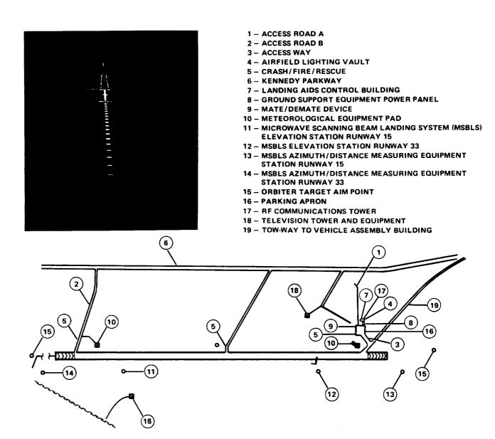
Figure 6-16.—Shuttle Landing Facility at KSC (108-KSC-376C-42/23).
