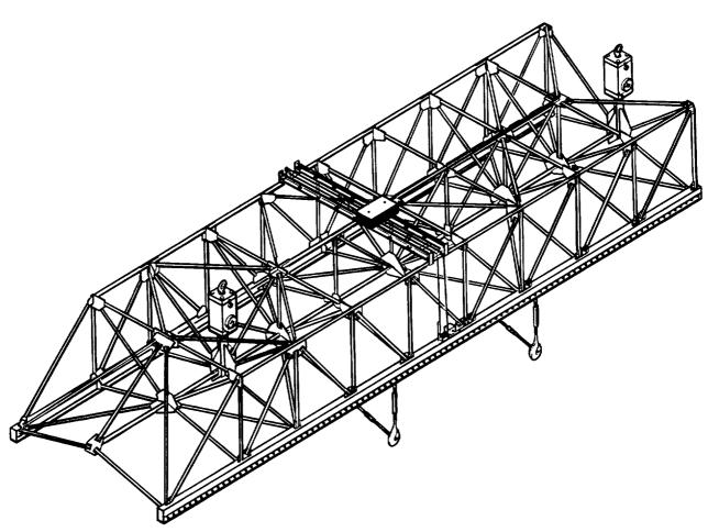
Figure 6-14.—Payload strongback.
