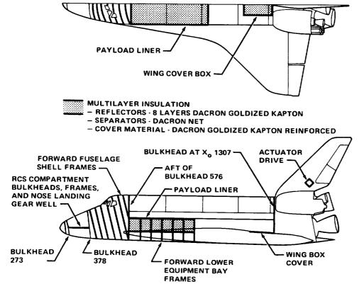
Figure 4-11.—Orbiter passive thermal control system.
