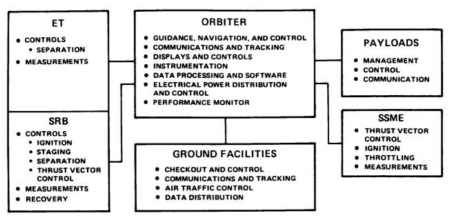
Figure 4-13.— Orbiter avionics system.
