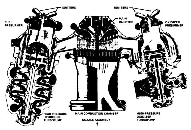
Figure 2-4.—SSME powerhead component arrangement.
