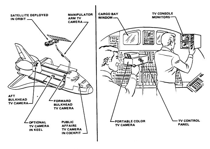
Figure 4-17.— Orbiter closed-circuit television system.
