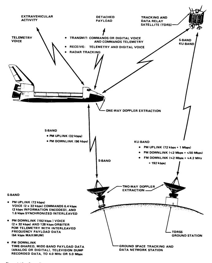
Figure 4-16.—Space Shuttle orbital communications and tracking links.
