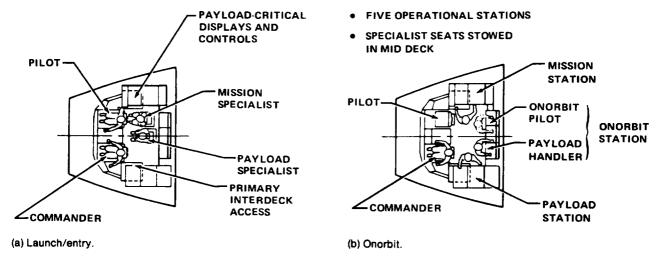
Figure 3-5.—Flight-deck crew cabin arrangement.
