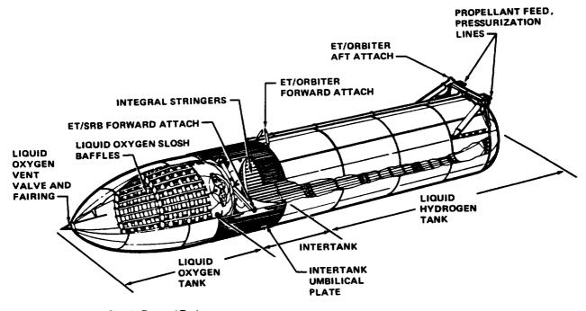
Figure 2-17.—Space Shuttle External Tank.
