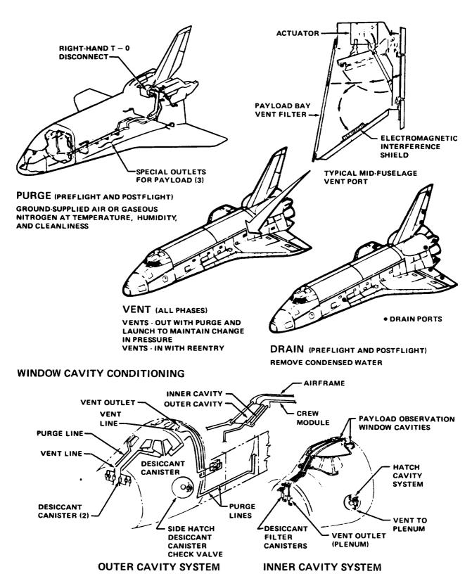
Figure 4-12.— Orbiter purge, vent, and drain system.
