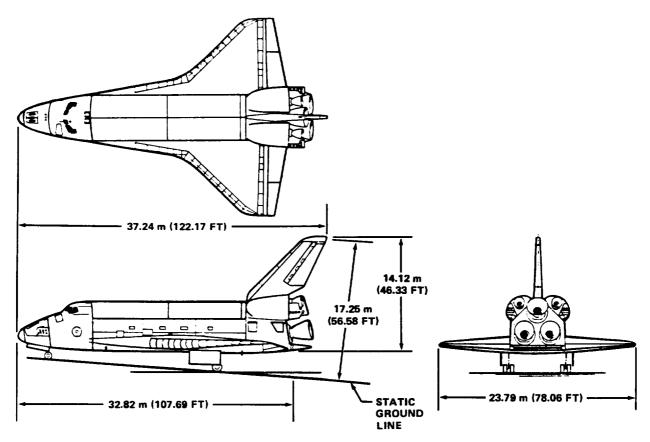
Figure 3-2.— Dimensions of the Orbiter vehicle.
