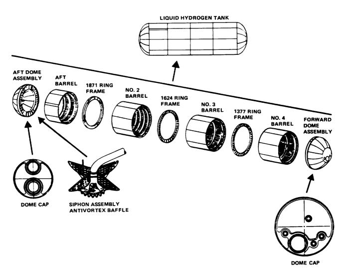
Figure 2-19.—ET liquid hydrogen tank structural assembly.
