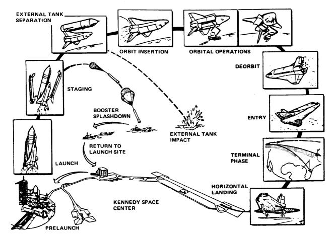
Figure 1-4.— A Space Shuttle typical mission profile.
