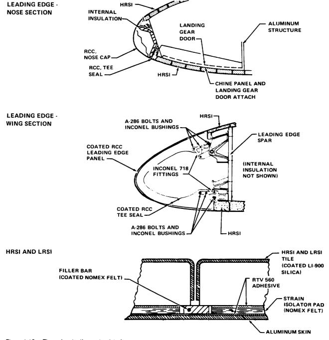
Figure 4-10.— Thermal protection system interfaces.
