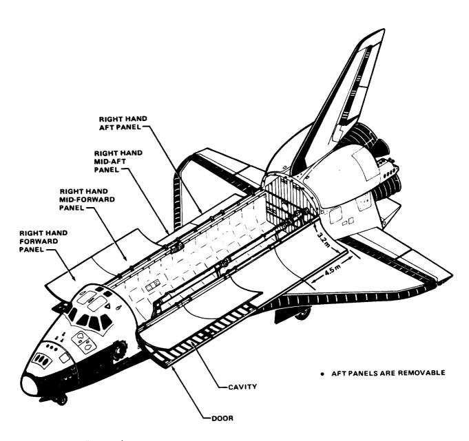
Figure 4-7.—Orbiter radiator panels.
