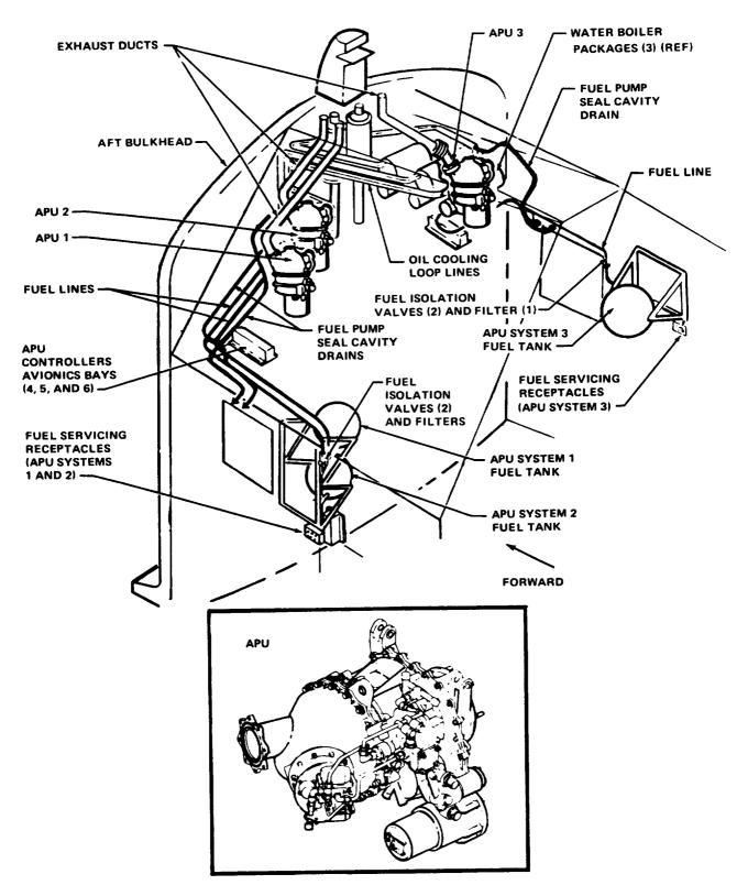
Figure 4-5.— Orbiter auxiliary power unit system.
