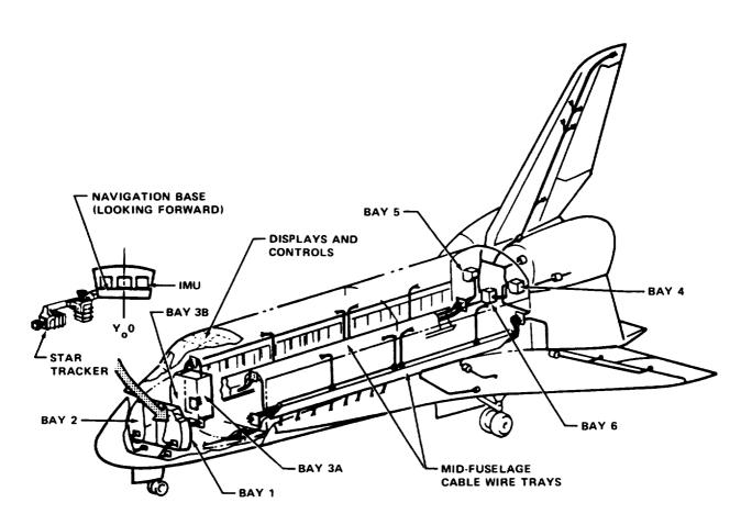
Figure 4-14.—Orbiter avionics system installation configuration.
