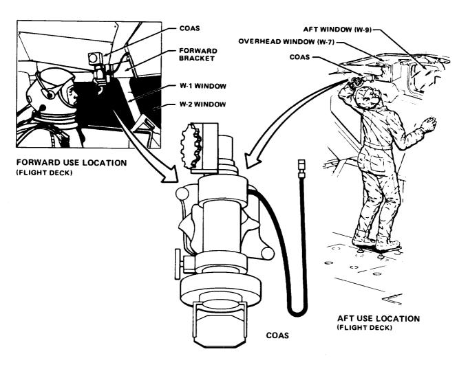
Figure 5-8.—Crewman optical alinement sight components and use locations.
