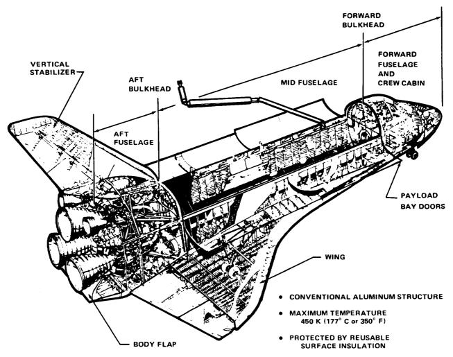
Figure 3-1.—Orbiter structures.
