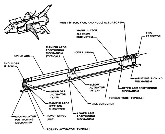
Figure 3-12.—Remote manipulator arm.
