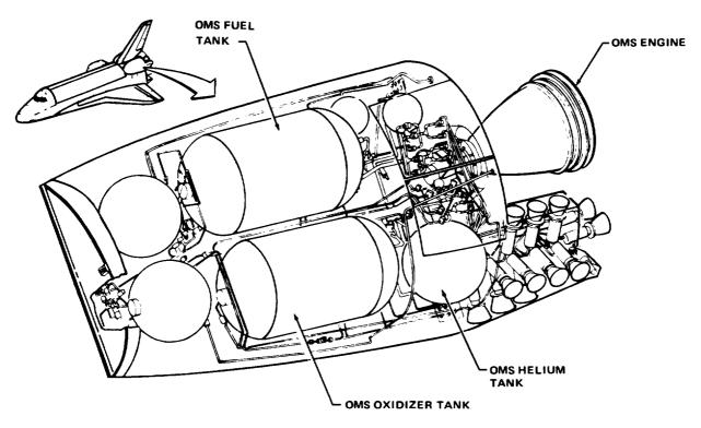
Figure 4-1.— Orbital maneuvering system.
