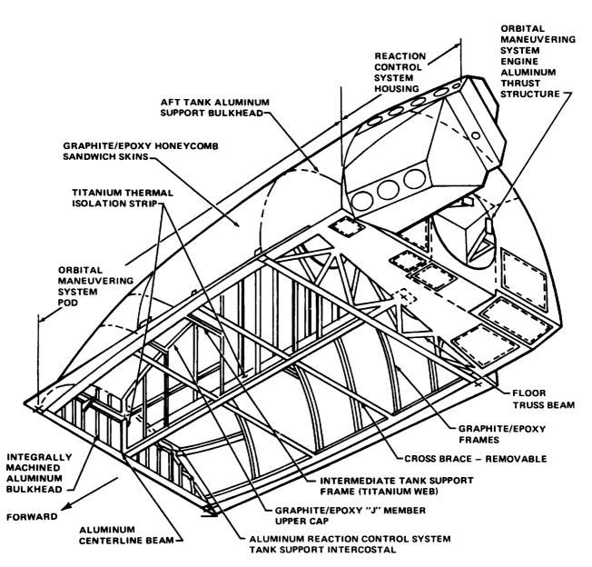
Figure 3-16.—Aft propulsion system thrust structure.
