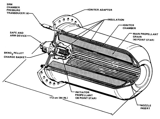
Figure 2-10.—Solid rocket motor igniter.
