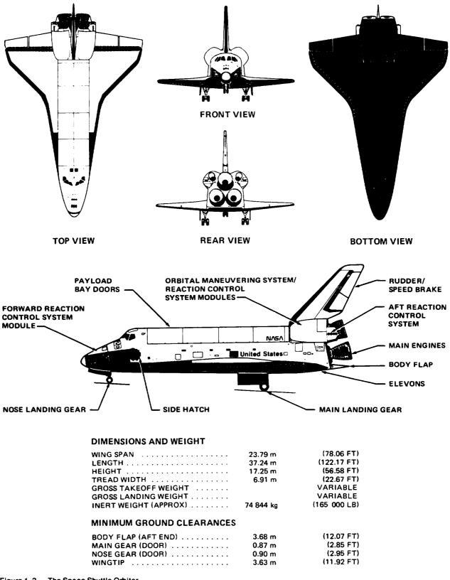
Figure 1-3.— The Space Shuttle Orbiter.
