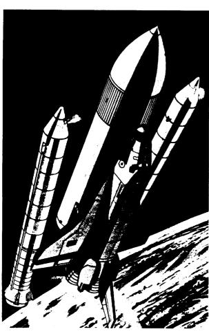
Figure 2-7.—Separation of Space Shuttle Solid Rocket Boosters (MSFC 003382).
