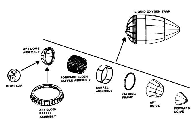
Figure 2-18.—ET liquid oxygen tank structural assembly.
