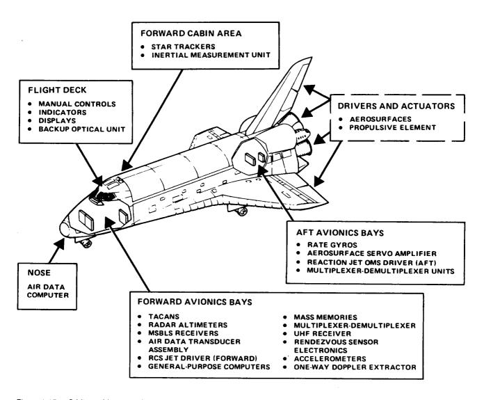
Figure 4-15.— Orbiter guidance, navigation, and control system.
