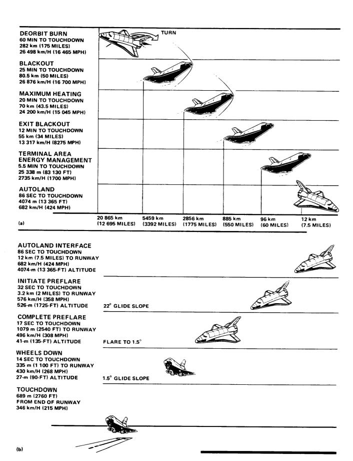
Figure 6-19.—Reentry burn cycle for the Shuttle.
