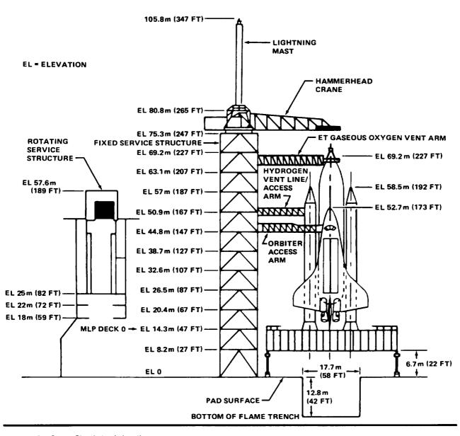
Figure 6-9.—Space Shuttle/pad elevations.
