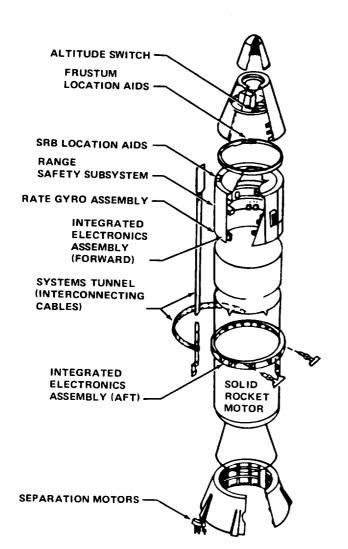
Figure 2-15.—SRB electrical system.
