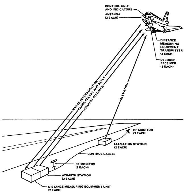
Figure 6-18.—Microwave scanning beam landing system.
